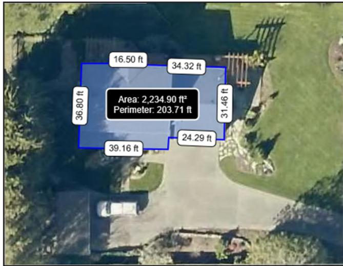
The “measure line” tool, from the same drop down menu, will allow you to get the lengths of property boundaries, roof lines, and other linear dimensions you might need to define for the project.
